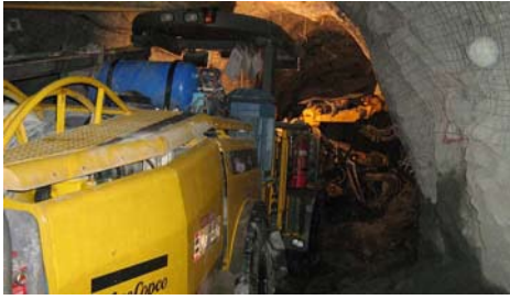
Mancala bought Atlas Copco Boomer M2D and 104 jumbos for mine development work at Costerfield in Victoria.
