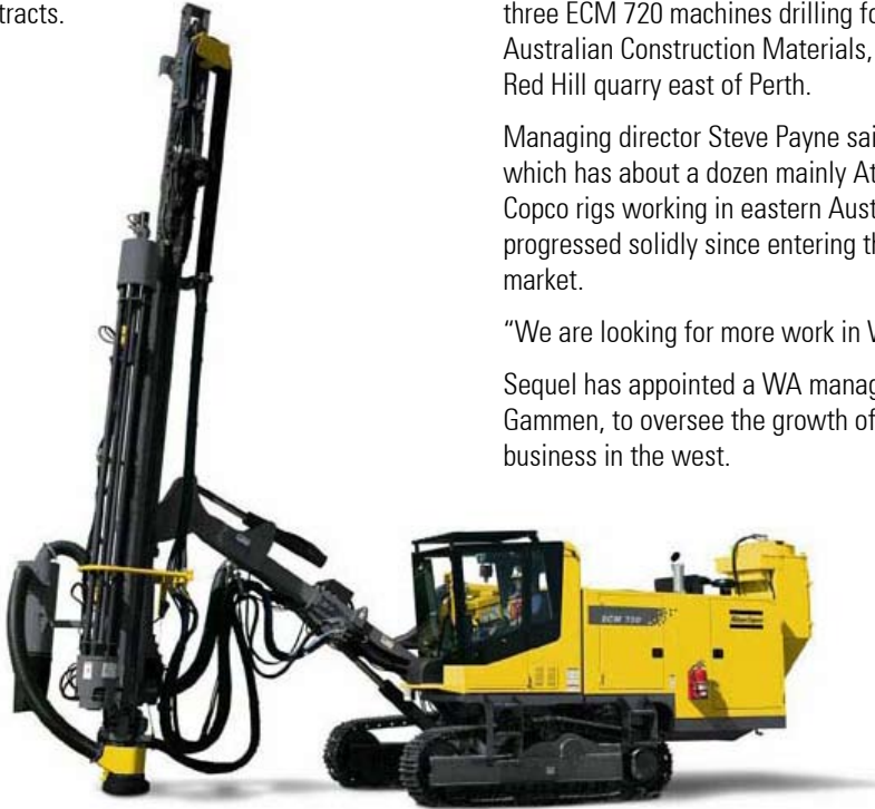
One of Sequel Drill & Blast's ECM 660 blasthole drill rigs.
