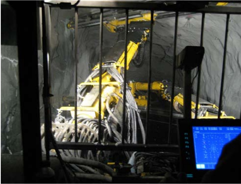
Window of opportunity ... Cadia East's Atlas Copco L2C30 development jumbo in action.
