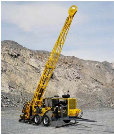
CS14 surface diamond drilling rig.
